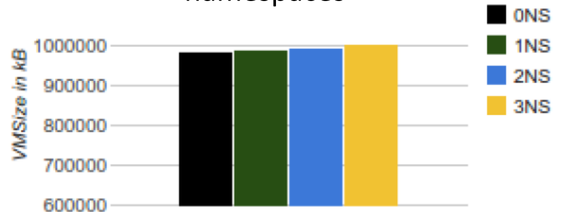
system_server process memory footprint vs. # namespaces
