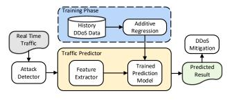
Fig. 1. Architecture of DDoSPVPredictor
