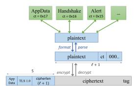
Figure 3. Constructing a TLS 1.3 record fragment
