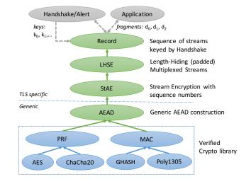
Figure 2. Modular structure of our proof. Green arrows denote security reductions proved by typing.
