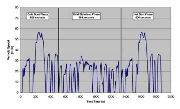
Fig. 1: FTP-75 (Federal Test Procedure) driving cycle depicting the speed over time. Image taken from EPA [20].
