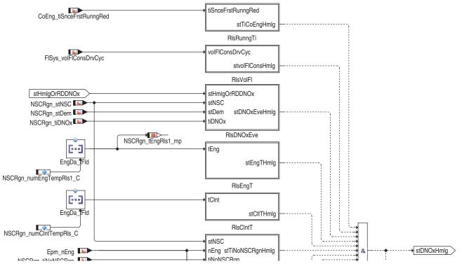
Fig. 12: Part of the NO<sub>x</sub> regeneration release logic "during homologation cycle" from function sheet EDC17C69 P 1264 for Fiat 500X. The homologation release signal requires multiple signals to be asserted, including stTiCoEngHmlg (Section IV-D). It is only asserted if engine running time does not exceed NSCRgn tiCoEngMaxHmlg C, set to 1600 seconds in the 55265162 Fiat 500X firmware image. Copyright Robert Bosch GmbH.
