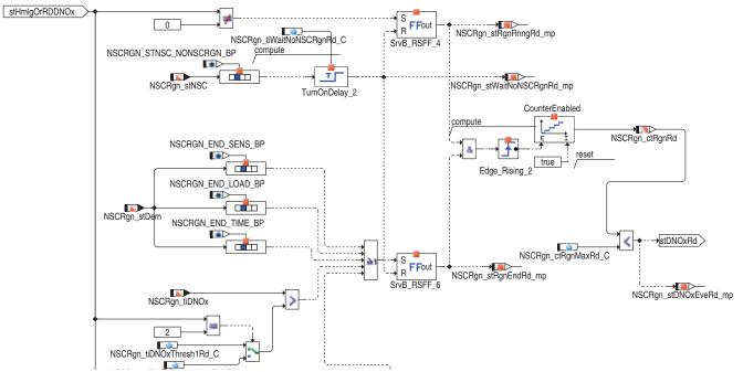
Fig. 13: Part of the  $NO_x$  regeneration release logic "during\_real\_driving" from function sheet EDC17C69 P 1264 for Fiat 500X. First element controls release based on engine running time. A parallel logic block controls release "during real driving." Copyright Robert Bosch GmbH.
