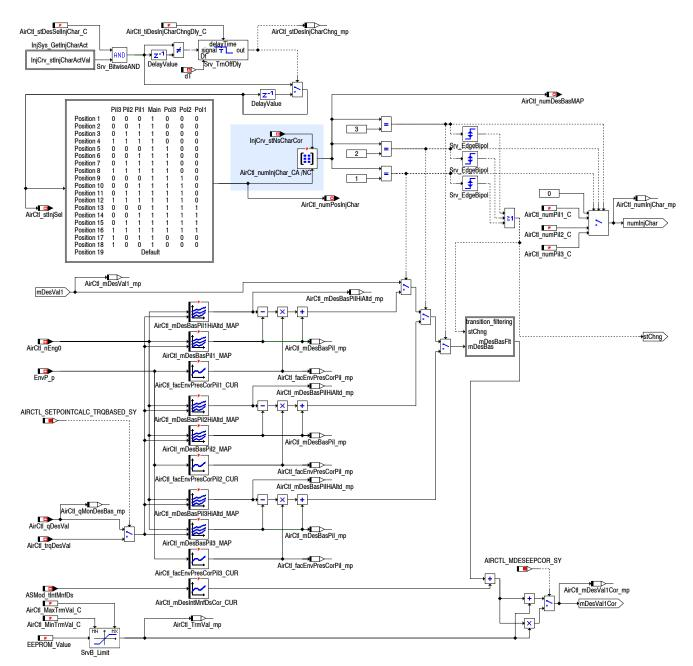
Fig. 11: Acoustic condition (signal InjCrv\_stNsCharCor) used to modify the desired air mass correction mDesVal1Cor, which modifies the desired air mass from which the amount of air recirculated is computed. AirCtl\_numInjChar\_CA is a two-dimensional array. The acoustic condition is used to select either row. From the EDC17C54 P 874 function sheet. Shading added by the authors. Copyright Robert Bosch GmbH.
