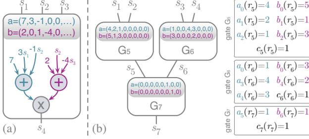
Figure 3. *Part (a)*: A bilinear gate representing the arithmetic function  $(7 + 3s_1 - 1s_2) \cdot (2 + s_2 - 4s_3)$  specified by coefficients  $a$  and  $b$ . *Part (b)*: A QAP for an arithmetic circuit with 4 input wires, 1 output wire, 3 bilinear gates. The circuit encodes the function  $f(s_1, s_2, s_3, s_4) = (4 + 2s_1 + s_2) \cdot (5 + s_1 + 3s_2) \cdot (1 + 4s_3 + 3s_4) \cdot (3 + 2s_4)$ . The non-zero equations for the QAP polynomials are shown on the right.
