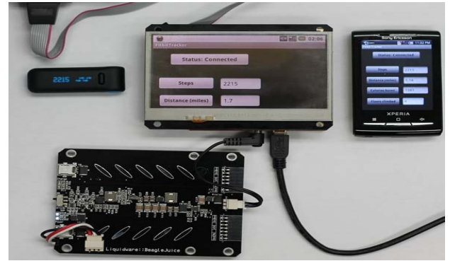
Fig. 3. Snapshot of testbed for FitLock, consisting of BeagleBoard and Xperia devices used as Fitbit trackers.
