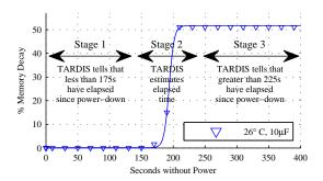
Figure 2: The TARDIS presents a three stage response pattern according to its amount of decay. Before 175 seconds, the percentage of bits that retain their 1-value across a power-off is 100%. For times exceeding 225 seconds, the TARDIS memory has fully decayed. The decay of memory cells between these two thresholds can provide us with a more accurate measurement of time during that period.
