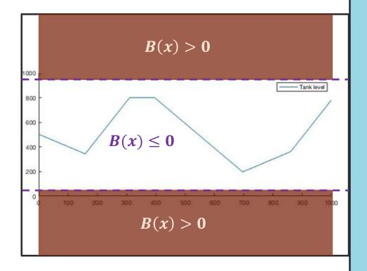
• Barrier function (B(x)) takes a positive value when the system is at unsafe region.
