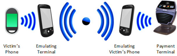
Figure 1: Overview of a Relay Attack
