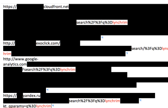
Fig. 3. The search term “lynchrim” is leaked in URLs (red text) to Google and Russia-based Yandex, and sometimes encoded in plain text in cookies.
