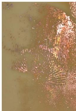
Fig. 10 Etched fingerprint remaining on PCB
