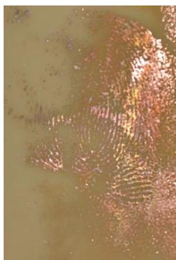
Fig. 10 Etched fingerprint remaining on PCB
