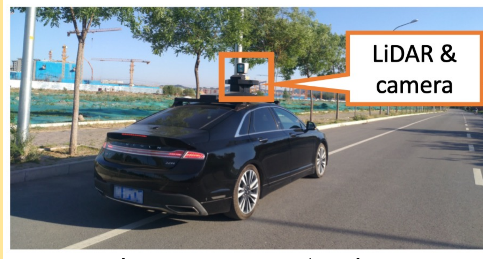
Road & car with LiDAR & camera
