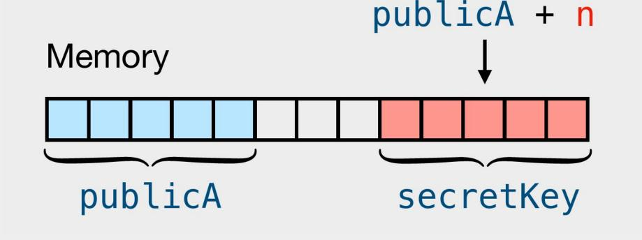
The example on the left is constant-time. But if the processor *misspeculates* into the branch, it can still leak bytes of secretKey via the cache!
