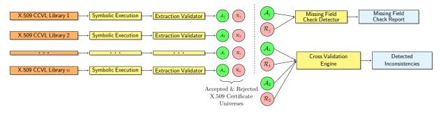
Fig. 1. Our noncompliance finding approach for X.509 CCVL implementations. **Symbolic execution engine** takes as input a CCVL implementation and extracts the approximated accepted and rejecting certificate universe whereas **extraction validator** validates it through concrete execution. **Missing field check detector** finds unscrutinized certificate fields from the universes. **Cross validation engine** performs cross validation among two implementations universes.
