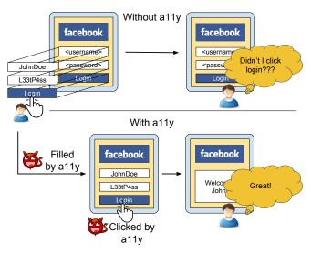
Fig. 4: This figure shows how our attack stealthily steals the user's credentials by using a fake UI and completing the login with the help of accessibility service vs. using only a fake UI (e.g., [11], [12], [1], [2], [3]).
