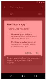
(b) This figure shows the warning message that is shown when the user clicks on the OK button that is covered by an overlay. The overlay in the figure is drawn semi-transparent for clarity. Of course, during a real attack, the overlay would be drawn completely opaque.
