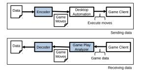
Fig. 1: Overview of data flow for sending an receiving in Castle. Shaded components are implemented as part of Castle while the others use existing off-the-shelf software.
