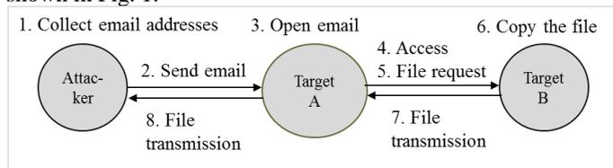
**Fig. 1. Process of an APT attack derived from our scenario**
