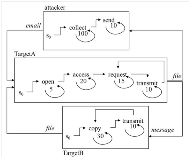
Fig. 2. Structure and state diagram of our APT attack model
