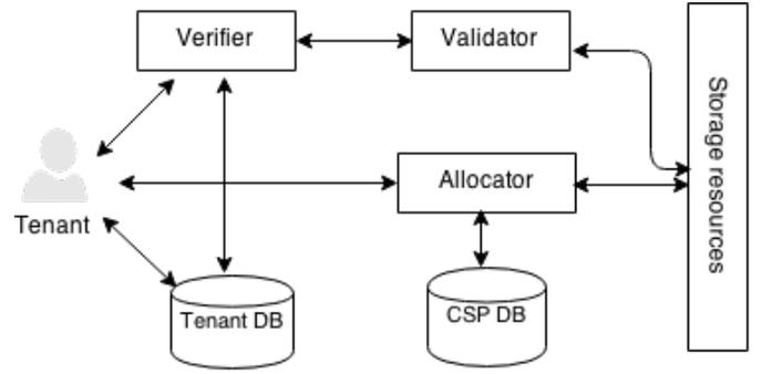
Fig. 2. Conceptual Assured Data Deletion(ADD) Architecture
