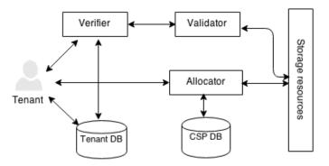
Fig. 2. Conceptional Assured Data Deletion(ADD) Architecture
