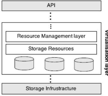
Fig. 1. A high level architecture of many layers that result from virtualization.
