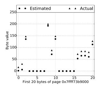
Fig. 7. Actual Bytes Estimation of a Nonzero Page in LIBC.
