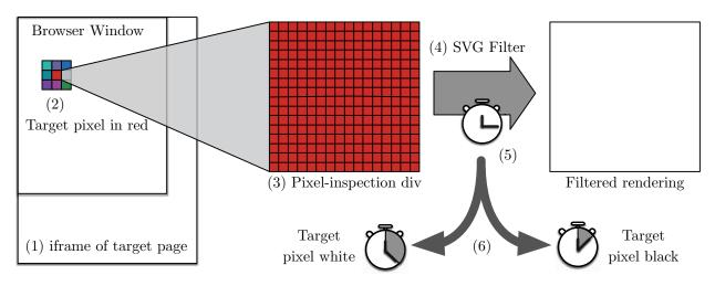
Figure 4: Cross-Origin SVG Filter Pixel Stealing Attack in Firefox
