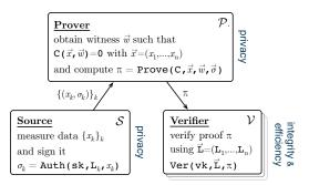
Figure 1. Three-party scenario in which a source S authenticates data  $x_k$ , and a prover  $\mathcal P$  proves to a verifier  $\mathcal V$  the satisfiability of a circuit C based on  $x_k$ . The source and the prover are interested in data privacy, whereas the verifier is interested in integrity and efficiency.
