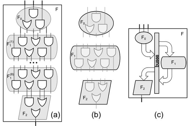
Figure 1: **MultiQAPs** (a) Most existing verifiable computation systems compile programs to a single large circuit-like representation, leading to internal redundancy. (b) By extracting common substructures, we can represent a program as an assembly of smaller circuits, but the verifier must now also check all connections between circuits. (c) MultiQAPs connect circuits using bus structures that support succinct and efficient commitments to the bus values.
