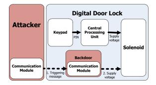
Fig. 2. The overview of power replay attacks: Dotted lines represent a malicious operation by attacker while solid lines represent a normal operation of door lock.
