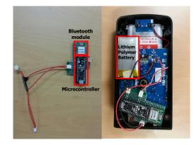
Fig. 3. Our prototype implementation for a power replay attack based on bluetooth (on  ${\tt Hyegang})$
