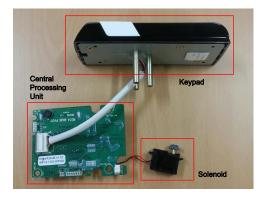
Fig. 1. An example of electronic door lock (made by Gateman)
