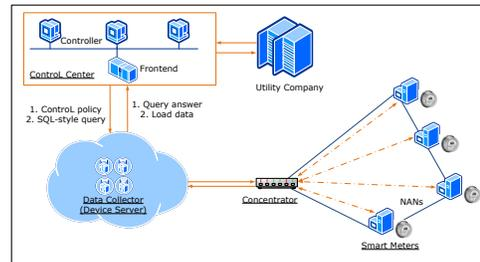
Fig. 1. Overview of the NAN based smart grid system.
