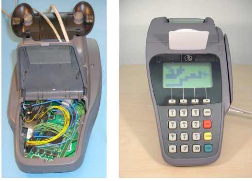
Figure 6. Modified Chip and PIN terminal, playing Tetris
