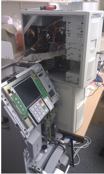
(a) Extracting disk image from NCR ATM
