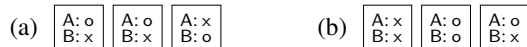
Fig. 1. Two ways of voting for the second candidate (candidate B) in the ThreeBallot protocol, where \times represents a marked position and \circ represents an unmarked position. All the other possibilities of voting for B can be obtained as permutations of these two.
