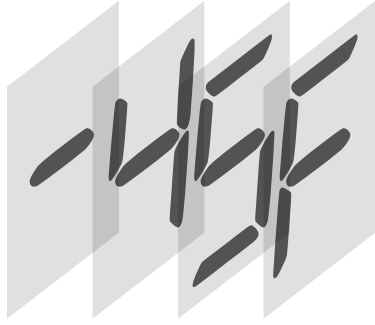
Fig. 3. 7-segment LCD symbols stacked to test three links per composite character. The - at the bottom is always visible, but the 4, 5, and F are only visible if a URL was visited.
